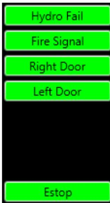
The inputs can be independently programmed using the setup window. They are usually programmed as emergency stops. If an input is activated, the input button will turn red and the simulator ride will not start. If a ride has already started and one of the inputs is activated, the machine will be put into emergency stop mode and it will return to the home position.
