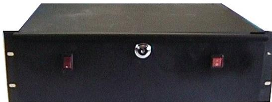
The control box is the interface between the computer and the motion simulator. The control box receives commands from the computer and sends them to the simulator. The control box also receives information from the simulator (emergency stop activations, cylinder positioning, etc.) and relays this information to the computer.
